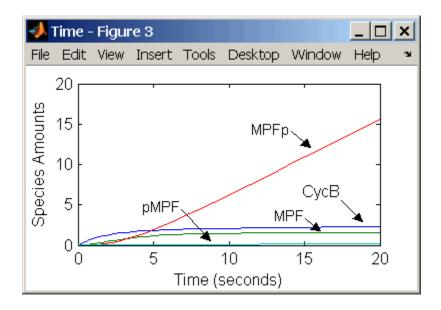
Test the simulation with Wee1p (inactive) = 0 and Wee1 (active) = 1.
