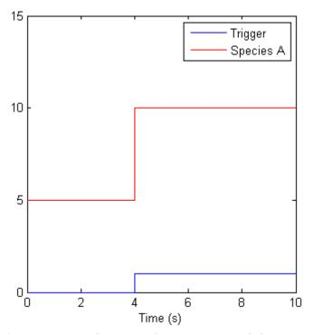
At time = 4 s the trigger becomes true and the event executes. In the figure above assuming that 0 is false and 1 is true, when the trigger becomes true, the amount of species A is set to 010. In theory, with a perfect solver, the event would be executed exactly at time = 4.00 s. In practice there is a very minute delay (for example you might notice that the event is executed at time = 4.00001 s). Thus, you must specify that the trigger can become true at or after 4s, which is time >= 4 s.
